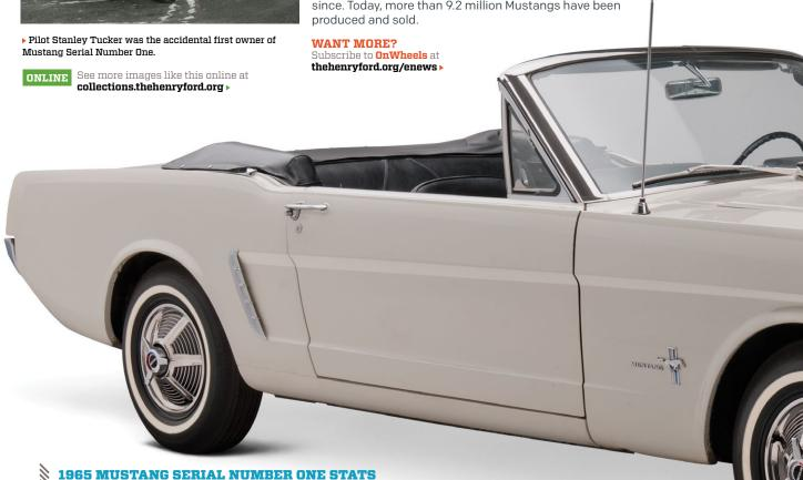
Engine: V-8, overhead valves, 260 cubic inches
