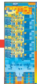
2012 3rd generation Intel® Core™ processor Initial clock speed: 2.9GHz Transistors: 1.4 billion Manufacturing technology: 22nm
